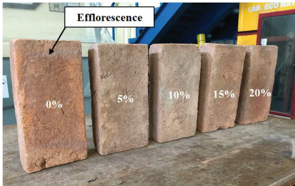
Figure 9. Efflorescence of brick specimens with different POFA contents.
